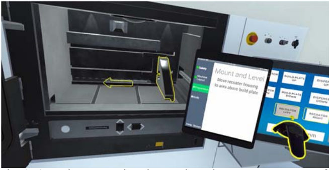
Fig. 1. A student operating the VR-based AM Training Tutor for the EOS M290 AM machine
